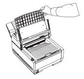
2. Check for paper jammed in the slot where received faxes or copies exit onto the document stacker. If you see paper
